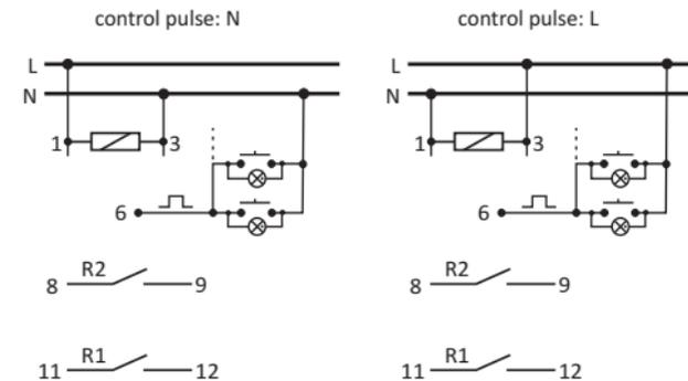
Example of relay installation with two lightning sections in „zero” (N) control system.
