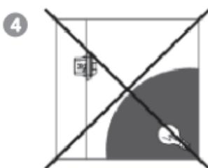
1. Do not mount near the outlet of an air conditioner or other heat sources.
