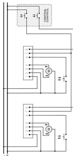
Example of wiring diagram for installation with two roller blind controller which work in common central control (control signal: N)
