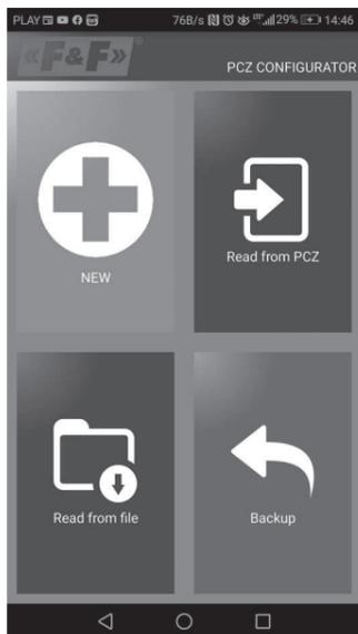
The function window allows to edit program as well as to load and save configuration to a PCZ controller. It appears automatically when we bring the phone closer to the controller, or when we create a new configuration. In the upper part of the screen the application displays a frame with following information:
