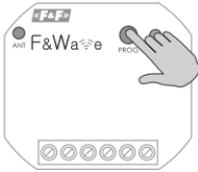
After the receiver is properly connected, press and hold the PROG button until the device activates output circuit and the communication LED will go off.
