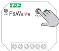
After the device is properly connected, press and hold the PROG button until the relay will switch on and the communication LED will go off.
