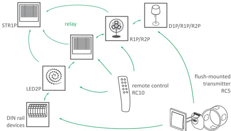
\* Range of up to 100 meters in open space without any interfering factors. In building conditions and in the presence of interference sources (power lines, transmitters, etc.) the actual range may be smaller.
