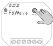
After proper connection, press and hold the PROG button until the circuit of the first channel will switch on and the communication LED will go off. To select a second channel for pairing, hold the programming button again until the circuit of the second channel switches on.
