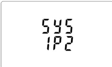
Use **P** and **MDI/PF/HZ** buttons to select the required system option: 1P2(W), 3P3(W), 3P4(W).
