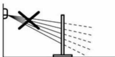
It is not recommended to mount the sensor in the vicinity of equipment that could alter the ambient temperature in a violent manner, for example radiators and air
