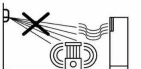
The sensor should be mounted on a rigid surface, at a minimum height of 2.4 m
