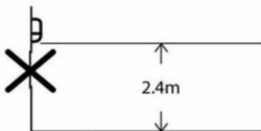
The motion sensor has a greater sensitivity to movement across the detection zone rather than in the direction of the sensor
