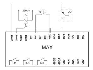
K – electromagnetic relay with isolated contact
