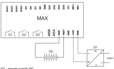
G1 - power supply DC G2 - gel battery 12V
