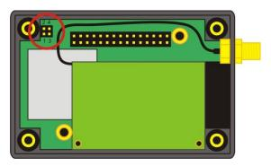
Location and pin numbers of the SPK output pin switch.
