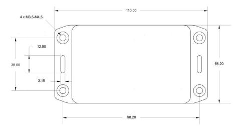
Dimensions of the controller and mounting holes
