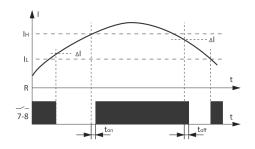
In this function, the relay operates in the so called "measuring window".
