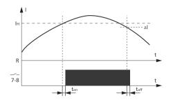
If the current in the measuring circuit exceeds the "Hi" setpoint, the relay contacts 7-8 will close and the contacts 9-10 open.
