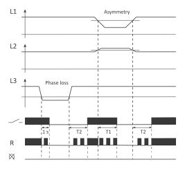
Legend: T1 = 1÷10 s T2 = 1÷60 s If a voltage drop below 150 V or a rise above 280 V is detected, the relay will be switched off with a delay of 1 s. In this case, both LEDs will will be switched off. If the phase voltages return to normal values, the relay will be switched on after T2 time.
