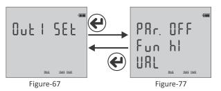
Parameter (PAr), Function (Valued) and Value (VAL). Press the right key to move the point (.) to the parameter. Press the down key to bring up the desired parameter. Then press the right key to move the point (.) to the function. Press the down key to set the function to low or high set. Press the right key to move the point (.) value. Press the down key
