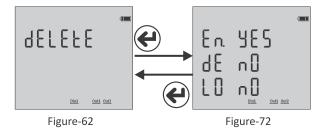
records here. Energy (En), Demand (dE) and Event logs (LE). Press the right key to move the point (.) to the record which you want to delete. Then press the down key to change the value to "yes". The record value which you do not want to delete must remain in "no".
