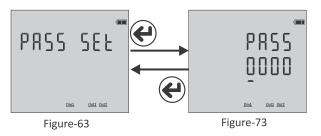
In order to pass through steps; press the button on the right. In order to change the value of the step press the, "down" button. You can change the step value with underline. If you press the set key after entering the password, the password is saved and the screen comes in Figure-63. Pressing the right key; you can pass through the parameters in the menu or pressing, "Esc" key; you can quit the menu.
