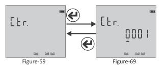
to the screen. Press right button to move between digits. Press the down key to change the value of the digit. You can change the digit value which is the underline. When
