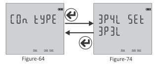
screen. It supports 2 types of connection like 3P4L (3 phase current 3 phase voltage neutral) and 3P3L (3 phase current 3 phase voltage without neutral). The link that says "Set" is acceptable. Press the right key to change the connection type. After the connection type is selected, When you press the key, it is saved and the screen comes in Figure-64. Pressing the right key; you can pass through the parameters in the menu or pressing, "Esc" key; you can quit the menu.
