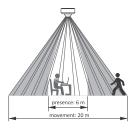
The direction of movement in the detection area
