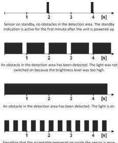
Signalling that the acceptable temperature inside the sensor is exceeded. Sensor operation is blocked until the fault has been removed. Too high temperature can be caused by connecting a too high load to the sensor.
