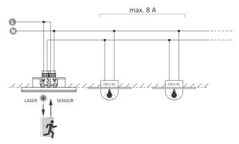
When it is necessary to control a load higher than 8 A, or a load with a high starting current, it is recommended to use external contactors or relays adapted to current surges (e.g. PP-1Z-LED 230 V). In this case, the DRL-60-230 switches an external relay to whose contacts the controlled load is connected.
