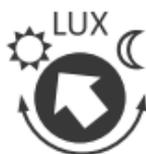
The sensitivity of the twilight sensor can be adjusted within the range of 3 lx to 2000 lx. Turning the control knob in the direction of the „moon“ icon will switch the light later, turning it in the direction of the „sun“ – will switch the light earlier. For the sensor to be active throughout the whole day, the control knob should be maximally turned in the direction of the „sun“.
