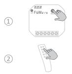
After the device is properly connected, press and hold the PROG button until the relay will switch on and the communication LED will go off.
