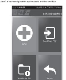
The function window allows to edit program as well as to load and save configuration to a PCZ controller. It appears automatically when we bring the phone closer to the controller, or when we create a new configuration. In the upper part of the screen the application displays a frame with following information:
