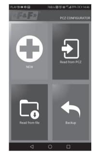
The function window allows to edit program as well as to load and save configuration to a PCZ controller. It appears automatically when we bring the phone closer to the controller, or when we create a new configuration. In the upper part of the screen the application displays a frame with following
