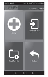
The function window allows to edit program as well as to load and save configuration to a PCZ controller. It appears automatically when we bring the phone closer to the controller, or when we create a new configuration. In the upper part of the screen the application displays a frame with following infor
