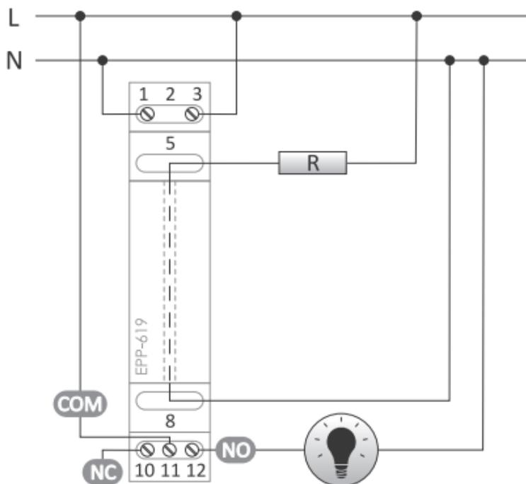
Example of a system for signalling the exceeding of the set current value
