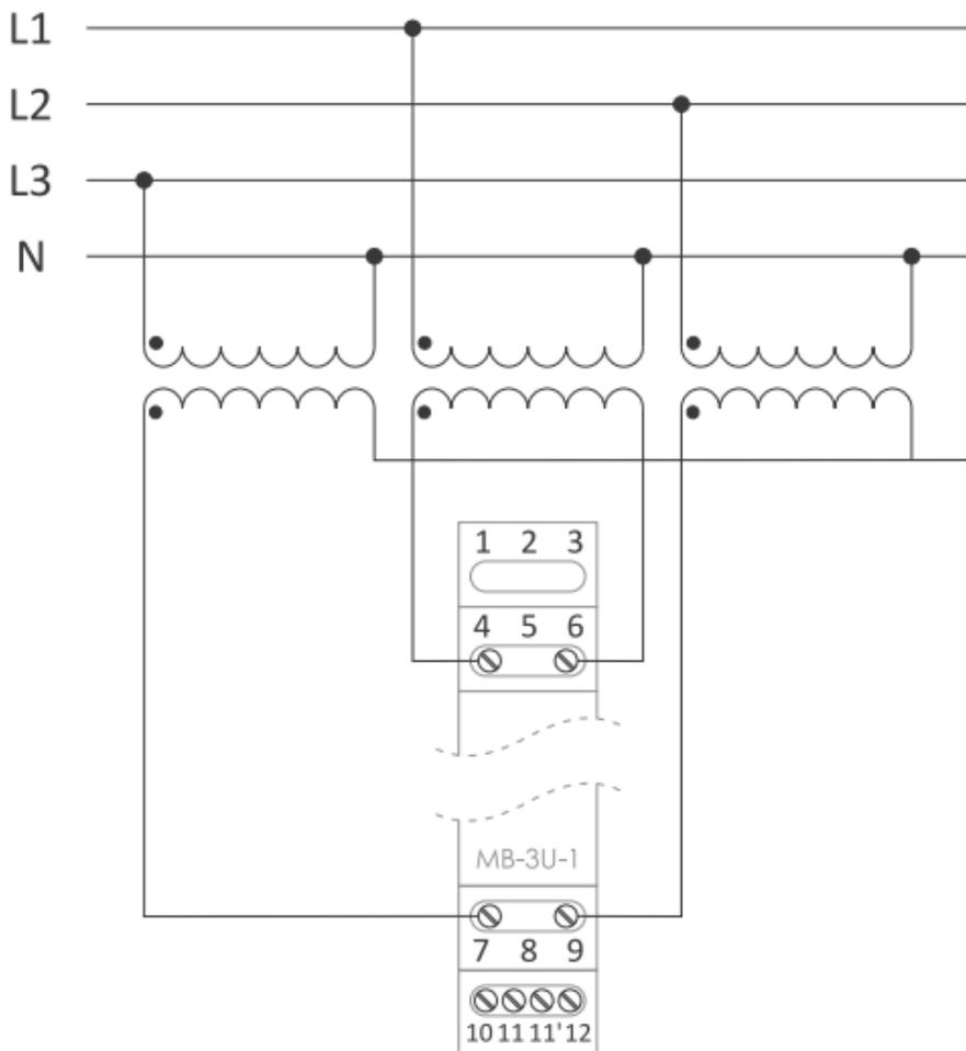
Indirect measurement of 3-phase network voltage
