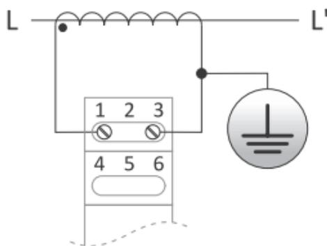
Indirect measurement of current using the current transformers
