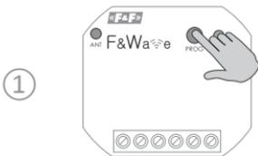
After you successfully connect the receiver, press and hold the PROG button until the device switches on the output circuit and the communication LED goes off.
