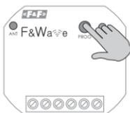
After you successfully connect the receiver, press and hold the PROG button until the device switches on the output circuit and the communication LED goes off.
