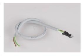
By default, a piece of three-wire cable is soldered to the sensors at the factory. The connection to the UTP / LIYCY cable should be made in the installation box by soldering and very thorough insulation. It is very important to correctly connect the sensors to the module (see table). Incorrect connection of the sensor (wire switch) results in damage to the sensor element.
