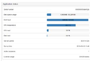
It allows displaying current information about the server and parameters of its current work status in the Dashboard module (similar to the Status tab).
