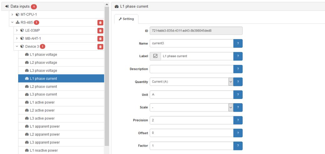
Expand the device segment and select the segment of the given parameter:
