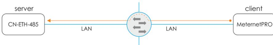
The MeternetPRO server initiates a connection to the converter with a static IP address.
