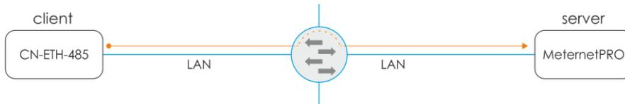
The converter initiates a connection to the MeternetPRO server with a static IP address.
