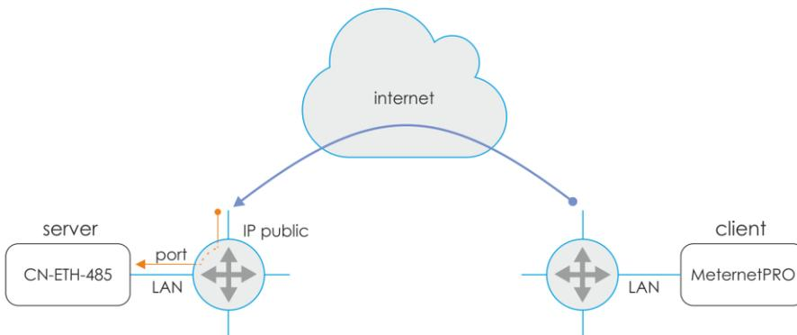
The MeternetPRO server initiates a connection to the converter to a public IP address for a location with the converter. Forwarding the request on the router to the designated communication port of the converter.
