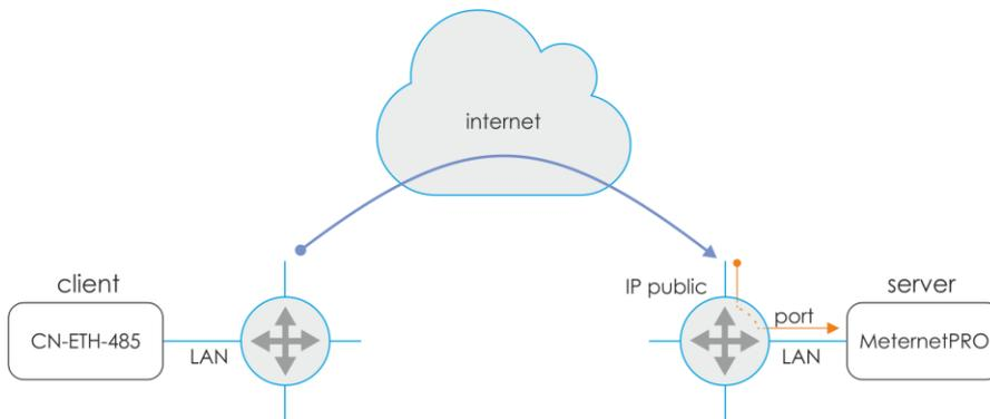
The converter initiates a connection to the MeternetPRO server to a public IP address for a location with the server. Forwarding the request on the router to the designated communication port of the MeternetPRO server.
