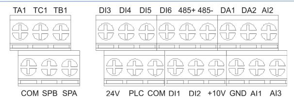
Figure 8) Terminal block for connection of control circuits (9KRSCB.V5 and above)
