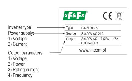
Figure 1) Rating plate of the inverter
