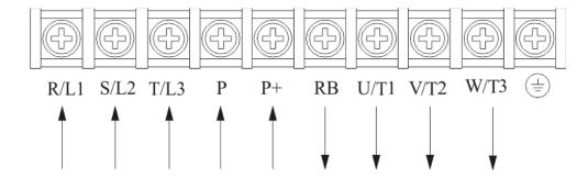
Figure 6) Terminal block to connect power circuits
