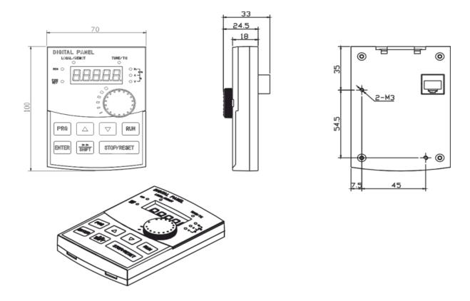
Figure 12) Operator panel – dimensions and mounting
