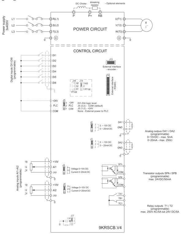
Figure 4) Wiring diagram (control board v4)
