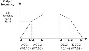
Acceleration – if the frequency is lower than the value **F7.14** then the acceleration is carried out according to the time F0.13 (first acceleration time). After crossing the frequency F7.14 the acceleration time switches to value F7.08 (second acceleration time).
