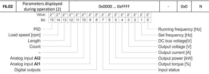
If any of the above parameters should be displayed during the drive operation, then 1 need to be set in the bit field corresponding to this parameter and then the whole number needs to be converted into a hexadecimal number (HEX) and in that form saved in parameter **F6.02**.
