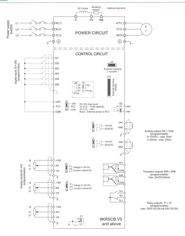
Figure 5) Wiring diagram (control board v5 and above)
