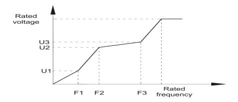
When programming the U/f characteristic keep the following relations between voltages and frequencies: V1 < V2 < V3 and F1 < F2 < F3
