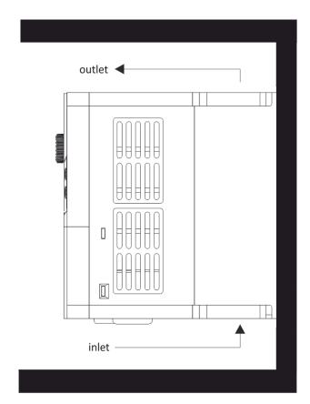
Figure 3) Example of the correct installation of the inverter
