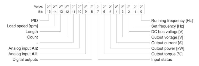
If any of the above parameters should be displayed during the drive operation, then 1 need to be set in the bit field corresponding to this parameter and then the whole number needs to be converted into a hexadecimal number (HEX) and in that form saved in parameter **F6.01**.
