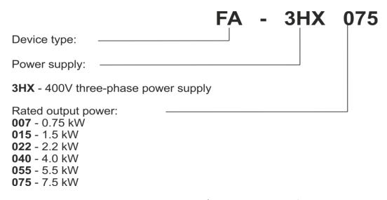
Figure 2) Inverter type identification
