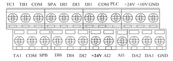
Figure 7) Terminal block for connection of control circuits (9KRSCB.V4)
