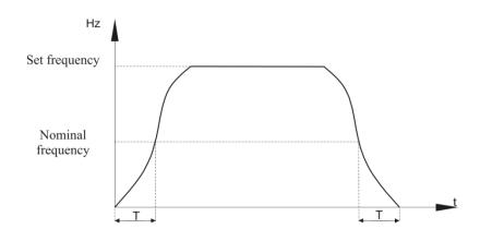
Acceleration/deceleration characteristic per second S curve
