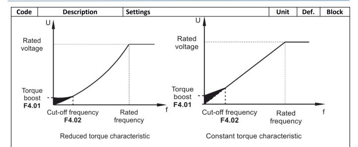
It is recommended to use a greater torque boost for heavy drives, where the standard driving torque is insufficient to accelerate the motor.
