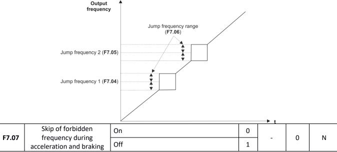
If **F7.07 = 0** then during acceleration and braking of the motor the output frequency will be able to pass through the zones of forbidden frequency (smooth change of frequency). If F7.07 = 1 then during start-up and braking the zones of forbidden frequency will be skipped, which also means that there will be a rapid frequency surge on the border of forbidden zone.
