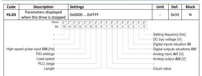
If any of the above parameters should be displayed when the motor is stopped, then 1 needs to be set in the bit field corresponding to this parameter and then the whole number needs to be converted into a hexadecimal number (HEX) and in that form saved in parameter **F6.03**.
