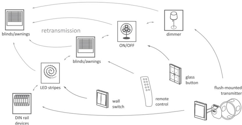
\* Range of up to 100 meters in open space without any interfering factors. In building conditions and in the presence of interference sources (power lines, transmitters, etc.) the actual range may be smaller.
