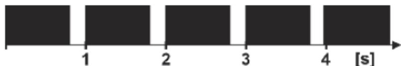
An obstacle in the detection area has been detected. The light was not switched on because the brightness level was too high.
