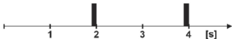
Sensor on standby, no obstacles in the detection area. The standby indication is active for the first minute after the unit is powered up.
