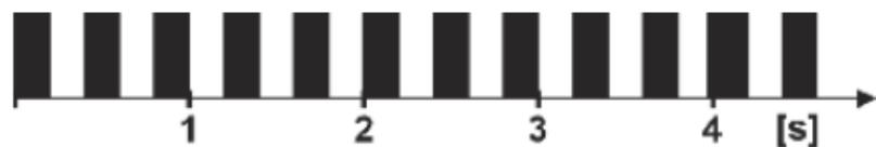
Signalling that the acceptable temperature inside the sensor is exceeded. Sensor operation is blocked until the fault has been removed.
