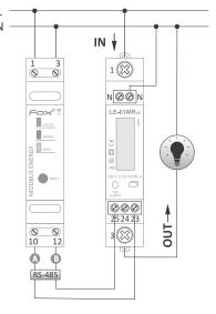
The connection scheme depends on the type of meter to be connected. Each time, the A-B communication outputs of the Modbus Energy integrator must be connected together with the A-B communication outputs of the energy meter. Example connection diagrams for all supported energy meters are available on the product page: www.fif.com.pl/fox/modbusenergy.
