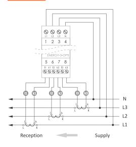
The correct type of measuring transformer must be set in the Fox application (for the Energy 3 module): **Module** settings → Measuring transformer.
