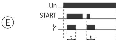
Generating a single pulse with time "t" by the rising edge of the START signal. During the time measurement, the system does not react to START pulses.
