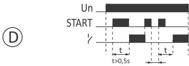
On delay of the relay using the START signal. When the relay is switched on, the next START pulse switches it off. The next START pulse causes the time to be measured again and the relay to be switched on. The interval between the trailing edge of the deleting signal and the rising edge of the START signal causing subsequent time measurement - minimum 0.5 sec.
