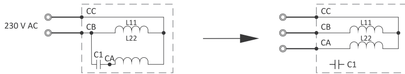
Typical single-phase motor diagram with starting capacitor
